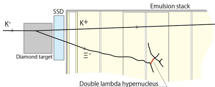
Fig. 1. A schematic diagram of the hybrid emulsion method for J-PARC E07.
