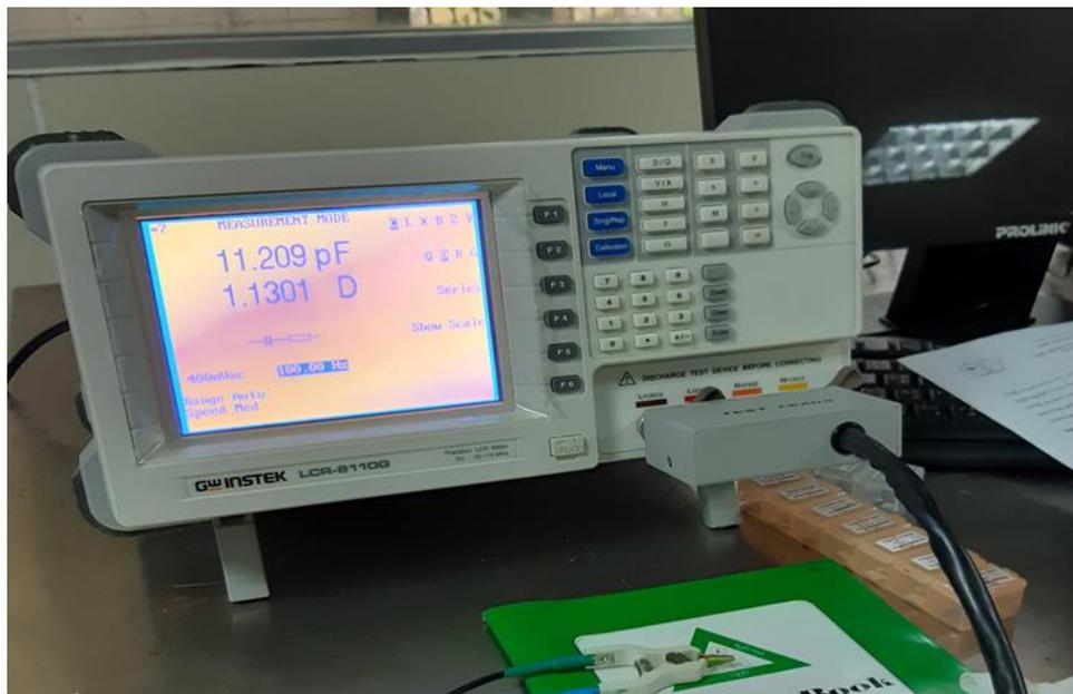
Figure 1 Capacitance-voltage measurement of the ceramics using LCR meter
