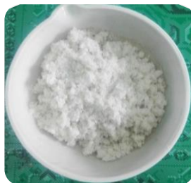
Figure 2 Prepared cellulose from oil palm bunch fiber
