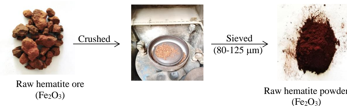
Figure 2. Powdering process in raw hematite ( \text{Fe}_2\text{O}_3 )
