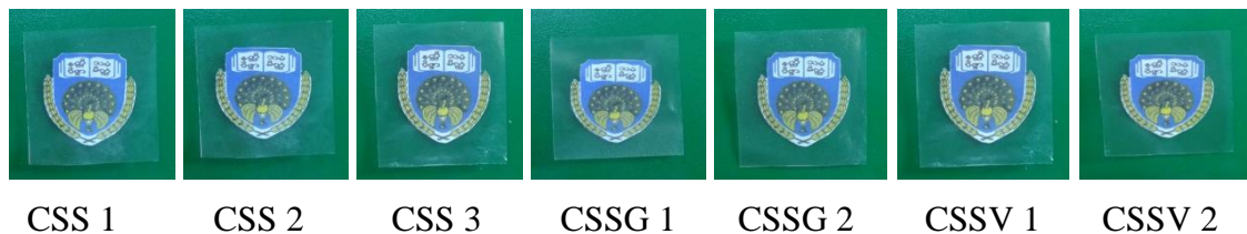
Figure 5. Transparency test of prepared bioplastics
