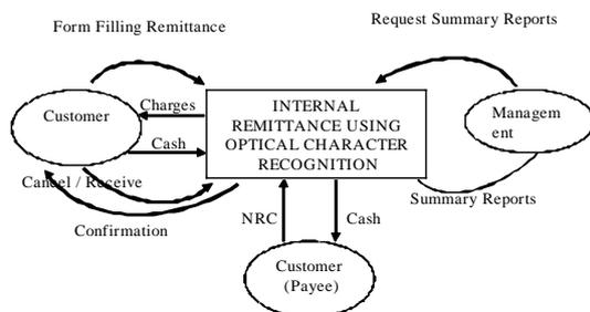
Figure 1. Context dataflow diagram of the system
