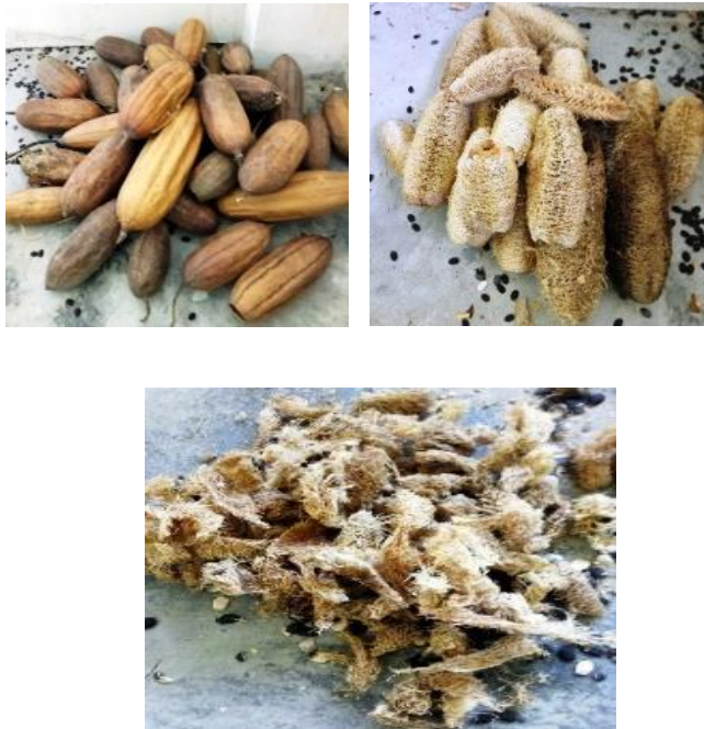
Fig.1 Luffa pod with skin, Luffa sponge and Chopped luffa fiber
