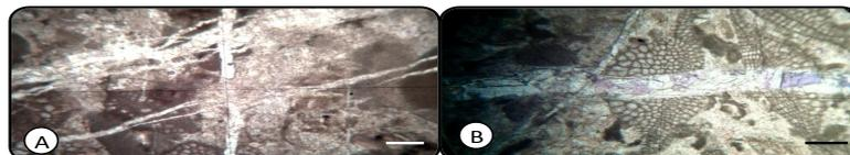
Fig.4 (A-B): Fractures of late stage calcite veins produced by equant blocky cement.
