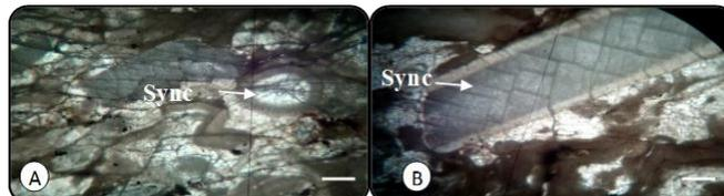
Fig. (8): (A) The syntaxial rim cement (Sync) found in bioclast. (B) Syntaxial cement can be clearly seen at the outside margin of bivalve spine. Scale bars are 0.1 mm.
