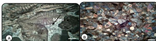
Fig. (5) (A):Meniscus fabrics (Meni) between the bioclasts and(B) Cemented mixture of sand sized quartz and rock fragments. Scale bar is 0.1mm.
