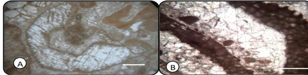
Fig. (3) (A): Twin planes crossing from grain to cement show syntaxial relationship. (B) The void filled with secondary pore-filling clear equant drusy spar. Scale bar is 0.1 mm.
