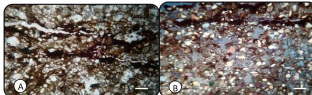
Fig. (11): Stylolite seams containing concentration of clay, iron minerals, organic matter and insoluble residues, scale bars are 0.1 mm.
