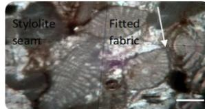
Fig. (10): Formation of foraminifera wackestone to packstone as a result of the closer packing and fracture of the grains, scale bar is 0.1 mm.
