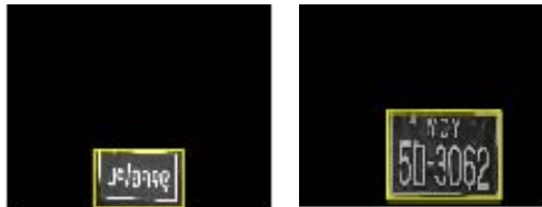
Fig. 10. Skew Angle Detection and Correction of the Images
