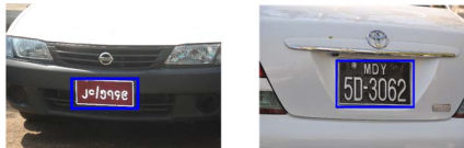
Fig. 11. Actual Number Plate Detection by Boundary Extraction
