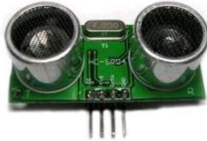
Fig.3 The HC SR04 ultrasonic sensor module
