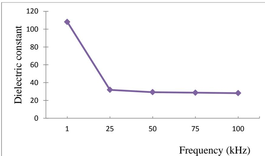
Figure (5a) Dielectric constant versus frequency of NiFe<sub>2</sub>O<sub>4</sub> sample
