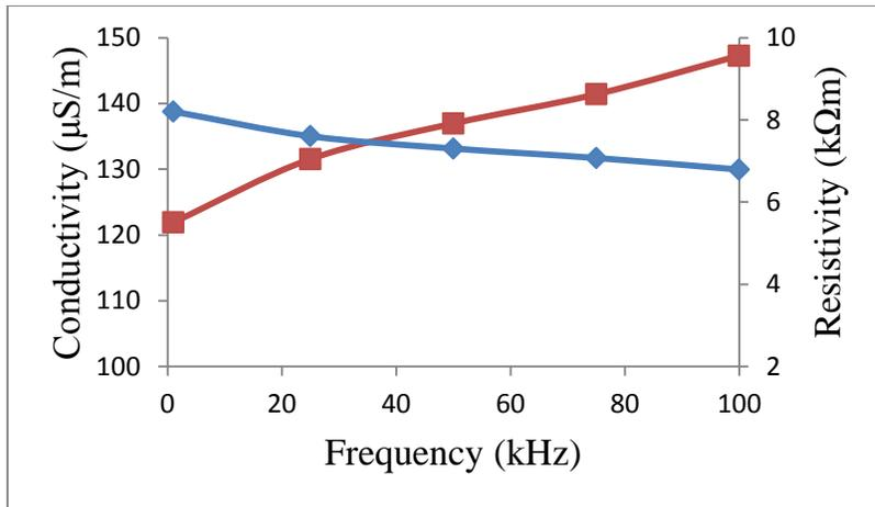
Figure (6) Resistivity and conductivity versus frequency of NiFe<sub>2</sub>O<sub>4</sub>
