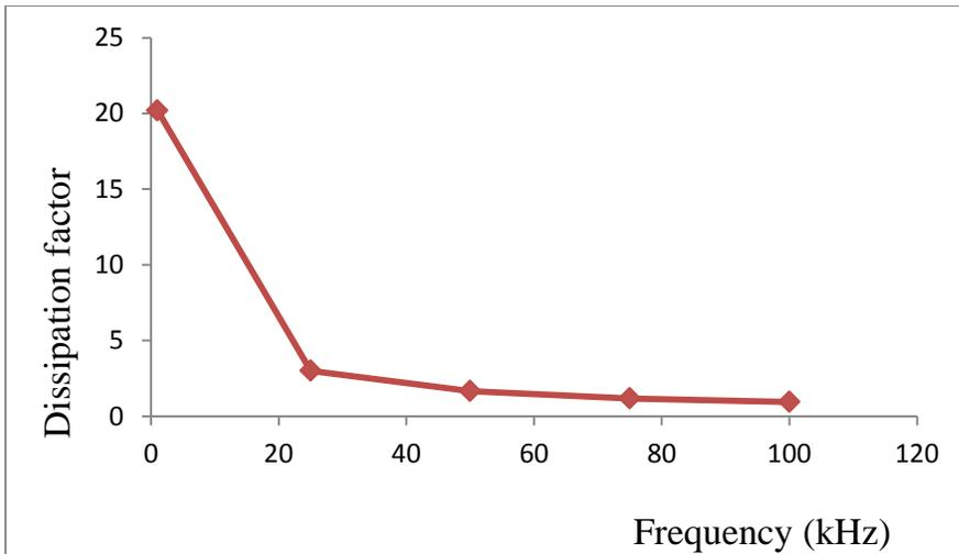
Figure (4) Dissipation factor versus frequency of NiFe<sub>2</sub>O<sub>4</sub> sample
