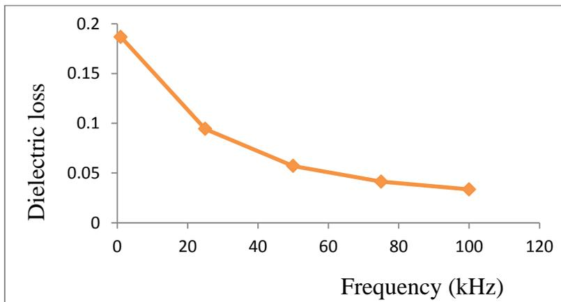
Figure (5b) Dielectric losses as a function of frequency of NiFe<sub>2</sub>O<sub>4</sub>
