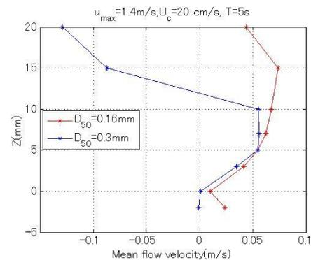
**Fig. 12.** Comparison of mean flow velocity between two types of sand ( $U_c = 0.2$  m/s)
