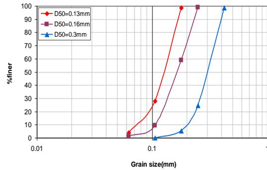
Fig. 2. Grain size distribution curves of the three sands in the experiments
