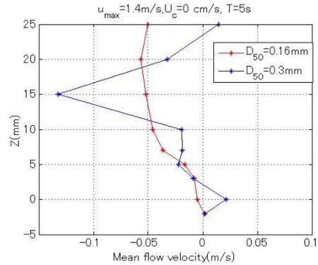
**Fig. 11.** Comparison of mean flow velocity between two types of sand ( $U_c = 0$  m/s)
