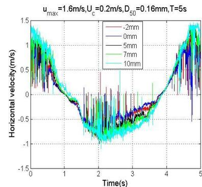
Fig. 9. Horizontal particles velocity for fine sand
