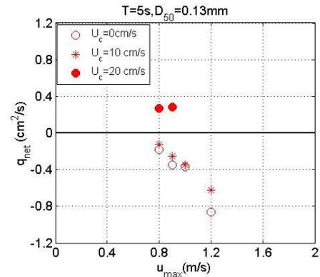
Fig. 5. Net transport rate as a function of flow velocity for very fine sand
