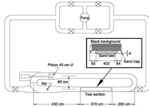
Fig. 1. Schematic diagram of the oscillatory flow tunnel (all dimensions are in cm)
