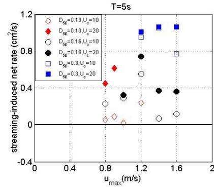
Fig. 8. Streaming-induced net transport rate as a function of flow velocity
