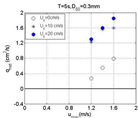
Fig. 7. Net transport rate as a function of flow velocity for coarse sand
