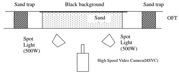
**Fig. 3.** Experimental apparatus utilized for image analysis (top view)
