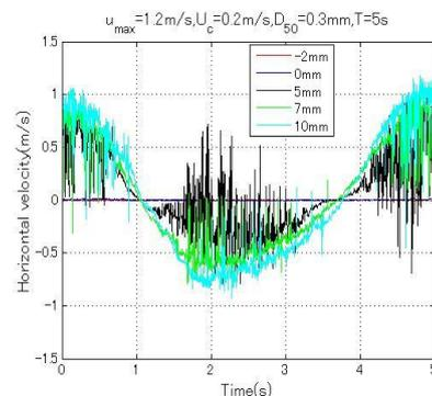
Fig.10. Horizontal particles velocity for coarse sand
