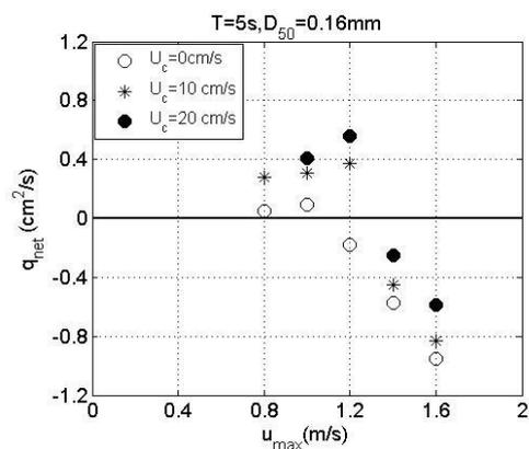
Fig. 6. Net transport rate as a function of flow velocity for fine sand
