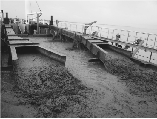
Fig. 3. Dredging ship and bottom material (mixture of sand and water) taken from Inner Bar (16° 45.817'N and 96°11.945'E) on 16 th September 2010.
