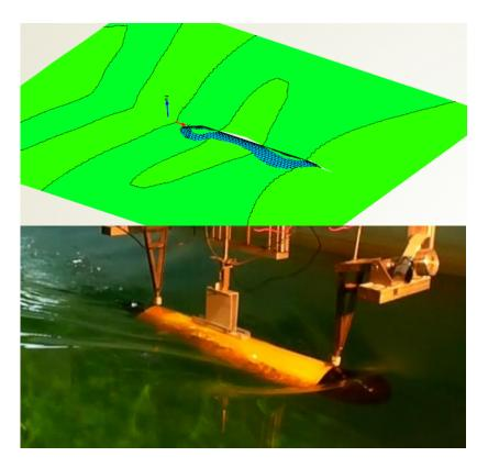
Figure 5(a). Towing tank test and CFD simulation with 1m/s
