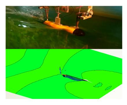
Figure 5(c). Towing tank test and CFD simulation with 1.8m/s
