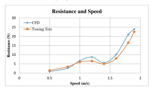
Figure 6 comparison of CFD and Towing test of ship resistance without appendages.
