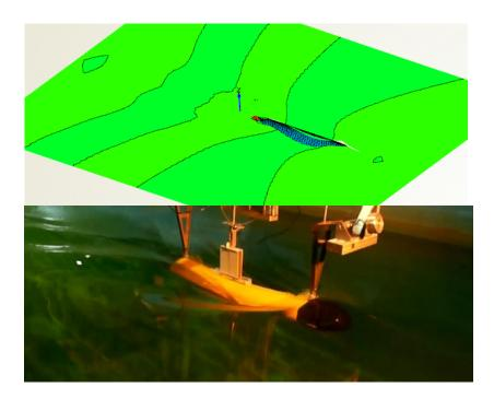
Figure 5(b). Towing tank test and CFD simulation with 1.4m/s
