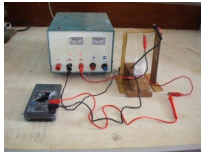
Fig.4 Experimental set up for electroplating system
