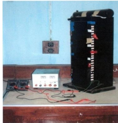
Fig.5 The measurement system of I-V characteristics
