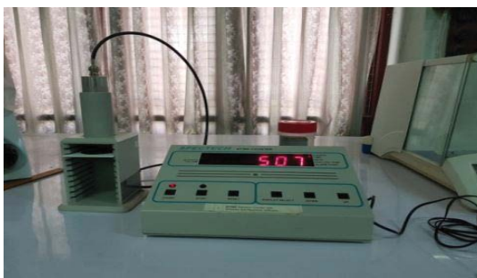
Figure 1 Experimental set-up of GM counter
