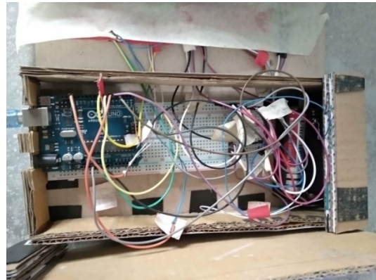
Figure5. Circuit connection of Arduino, Stepper motor and Servo motor
