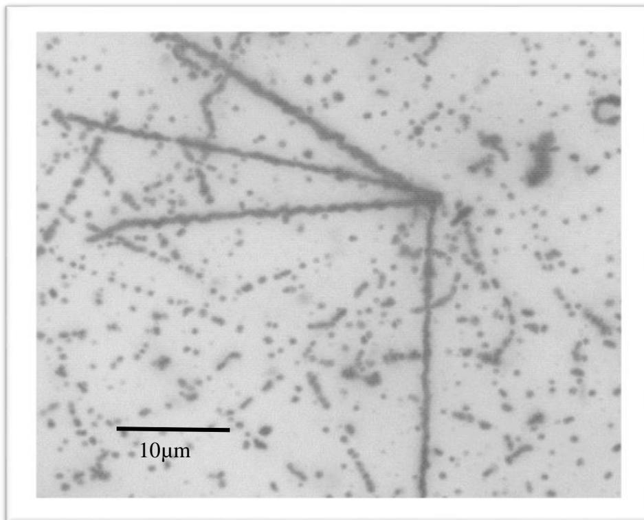
Fig. 3. A photograph of Uranium series in Nuclear Emulsion
