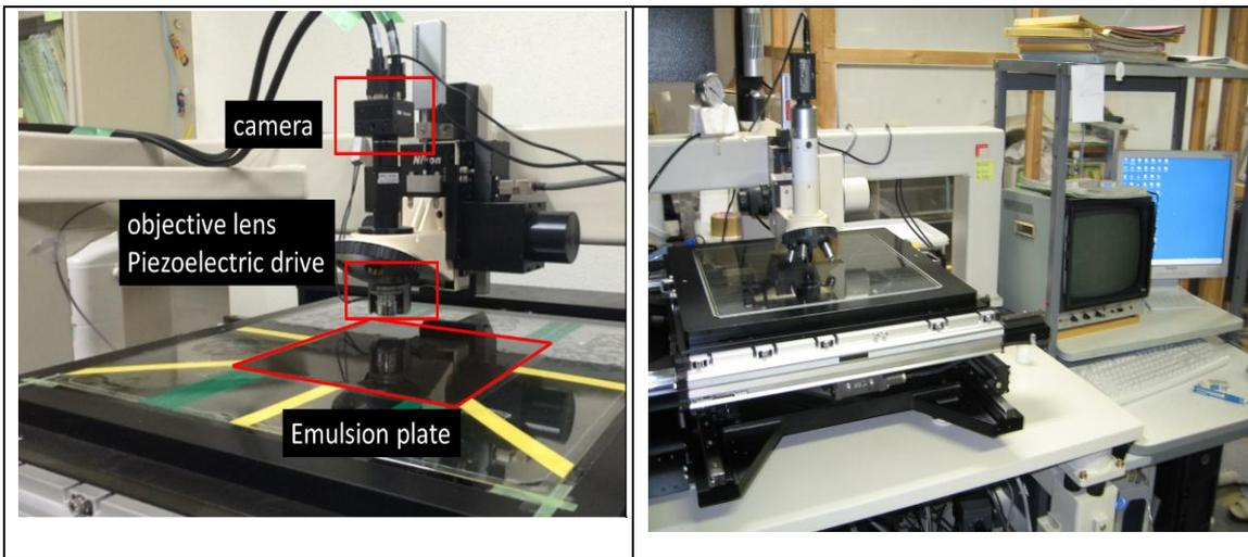
Fig. 4 Microscope systems for vertex picker and range measurement of charge particle tracks
