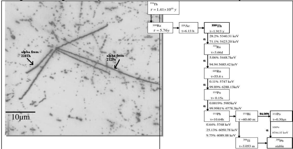
Fig. 2. A photograph of Thorium series in Nuclear Emulsion and decay chain
