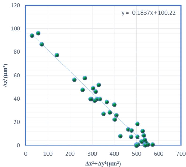
Fig. 6. The range distribution of  $\alpha$  particles as the scatter plots of  $\Delta z^2$  versus  $\Delta x^2 + \Delta y^2$  from the decay of  $^{228}\text{Th}$ .
