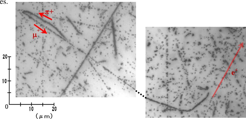
Fig. 1. The image of  $\pi^+ \rightarrow \mu^+ \rightarrow e^+$  event in nuclear emulsion of E373 experiment.
