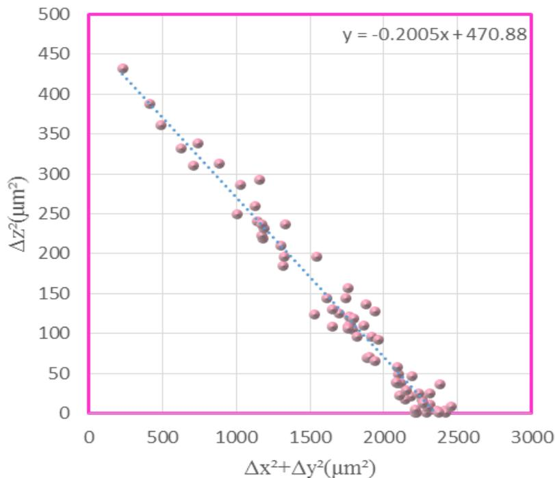
Fig. 5 The range distribution of  $\alpha$  particles as the scatter plots of  $\Delta z^2$  versus  $\Delta x^2 + \Delta y^2$  from the decay of  $^{212}\text{Po}$ .
