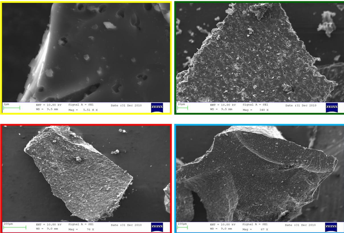
Fig. 6. SEM images after adsorption of heavy metal by four size CSC samples: Upper left = 120 mesh, Upper right = 90 mesh, Lower left = 60 mesh, Lower right = 30 mesh
