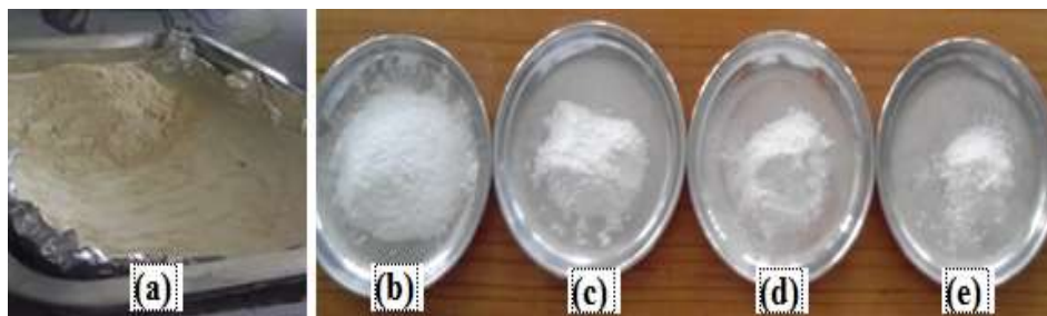
Figure 3: Natural Kaolin (a); Acid Activated Kaolin Prepared using Various Sulphuric Acid Concentrations (b) 2.5 M (c) 3.5 M (d) 4.5 M and (e) 5.5 M
