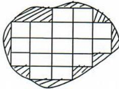
Figure 2-a. A typical geometry suitable for approximation with rectangular elements.
