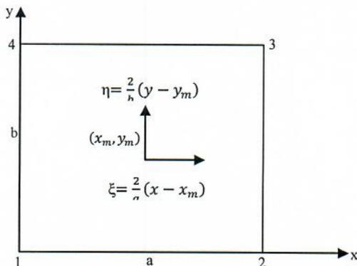
Figure 1. The four-node rectangle  $(x_m, y_m)$  are the coordinates of the mid-point of the rectangle
