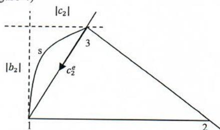
Figure 4. Boundary element with side 3-1 approximating the boundary
