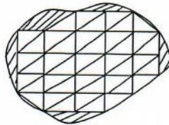
Figure 2-b. Approximation with triangular elements using the same number of nodes.
