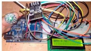
Fig. 13. Prototype of the heart rate monitoring system
