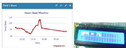
Fig. 14. Displaying the heart rate data in the graph form in ThingSpeak and on LCD
