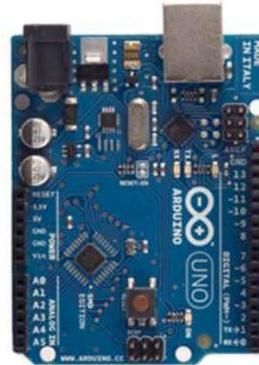
Fig. 3. Arduino Uno development board
