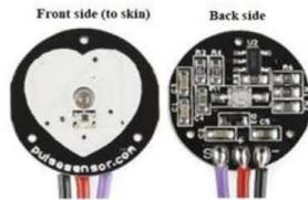
Fig. 4. Front and back side of pulse sensor
