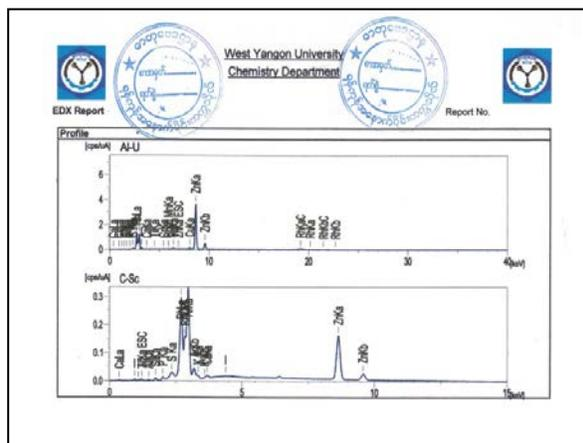
Fig. 7 EDX Pattern of ZnO NPs
