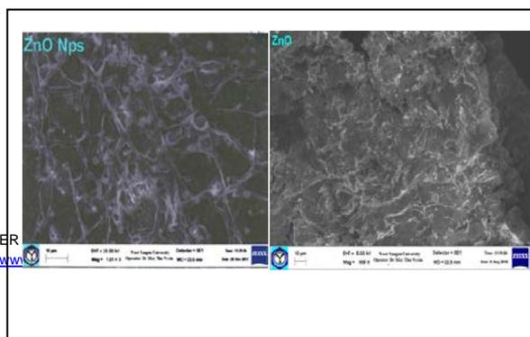
Fig. 6 SEM Micrograph of Zinc Oxide Nanoparticles
