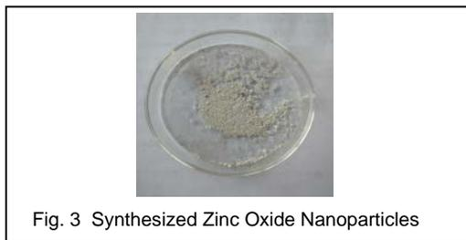
Fig. 3 Synthesized Zinc Oxide Nanoparticles
