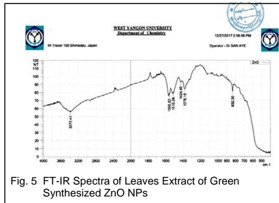
Fig. 5 FT-IR Spectra of Leaves Extract of Green Synthesized ZnO NPs
