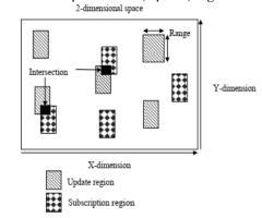
Figure 1: Example of region intersection in the 2dimensional space
