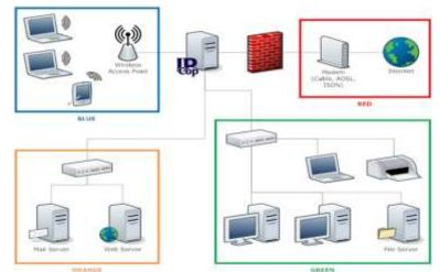
Fig -3: Four Types of Network Interfaces in IPCop
