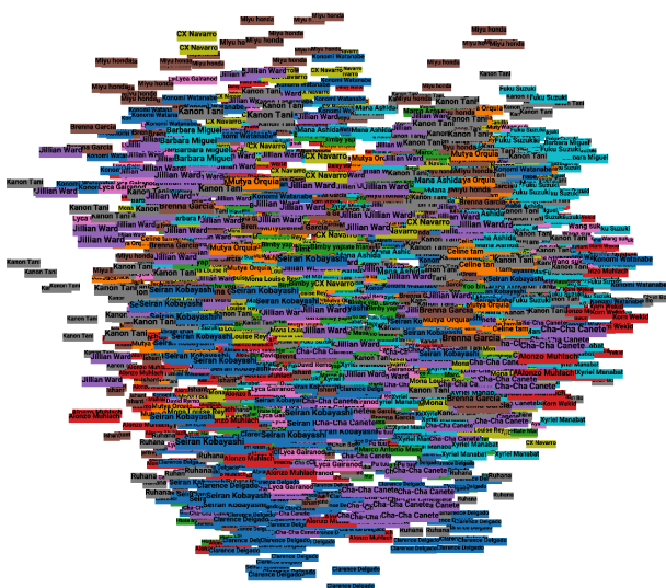
Figure 9. Embeddings which generate from FaceNet show as 3D graph. One color represents one class.
