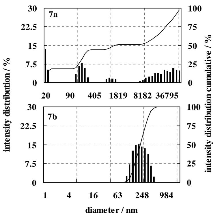
**Fig. 5.** Representative histogram of the particle size distribution for  $C_{12}Py^+$ -AFA system ( $1.5 \text{ mmol dm}^{-3} C_{12}Py^+$  and  $0.05 \text{ g dm}^{-3}$  AFA) at pH 9.18 and ionic strength 0.03M. (a) without  $C_{12}Py^+$ , (b) with  $C_{12}Py^+$ .
