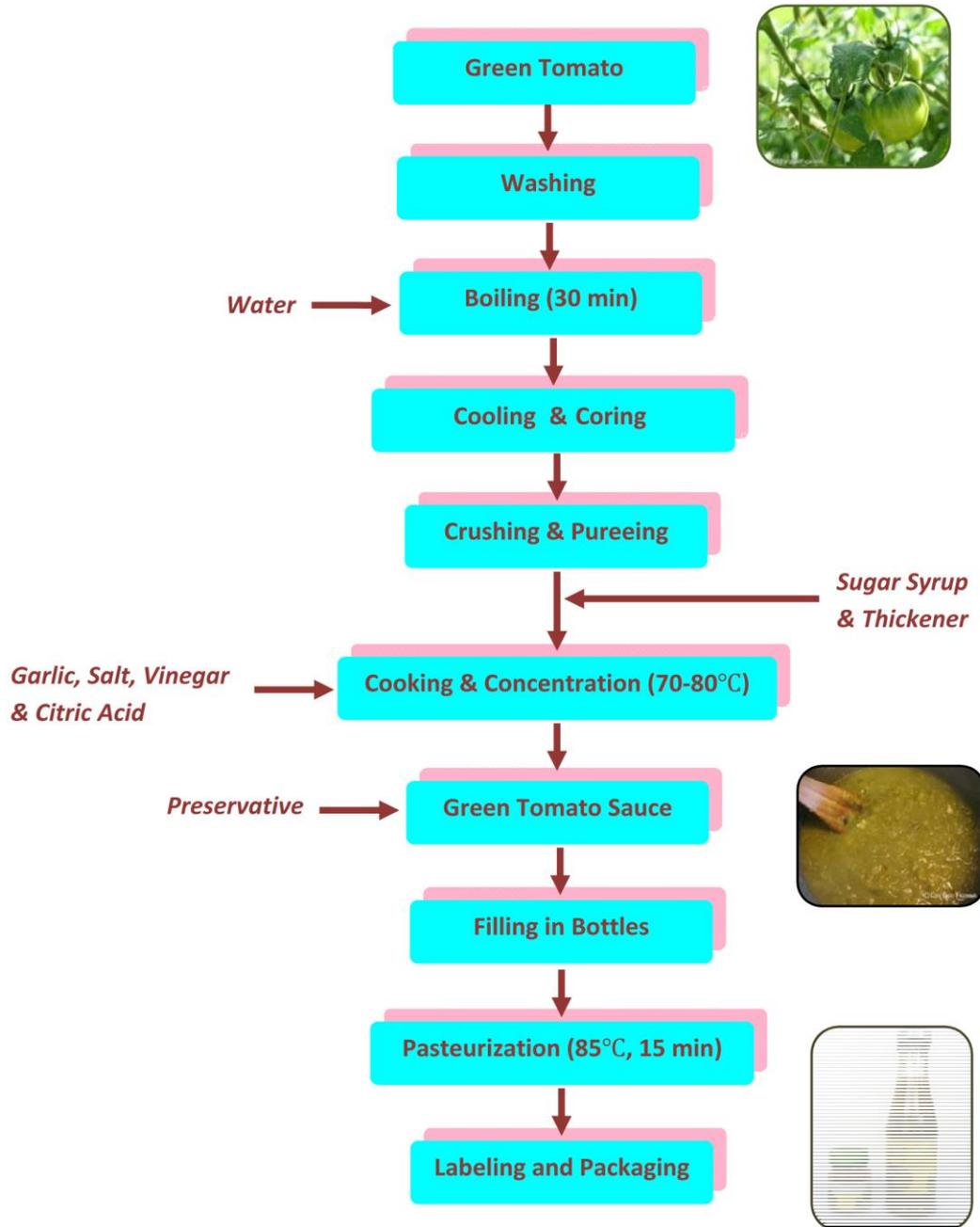
Figure( 8) Process Flow Diagram for the Preparation of Green Tomato Sauce
