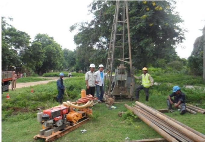
Figure 1.3 The SPT test in the site investigation at SG-1 near Sagaing Taungyo Road (N 21° 54' 25.7" and E 95° 59' 07.2")
