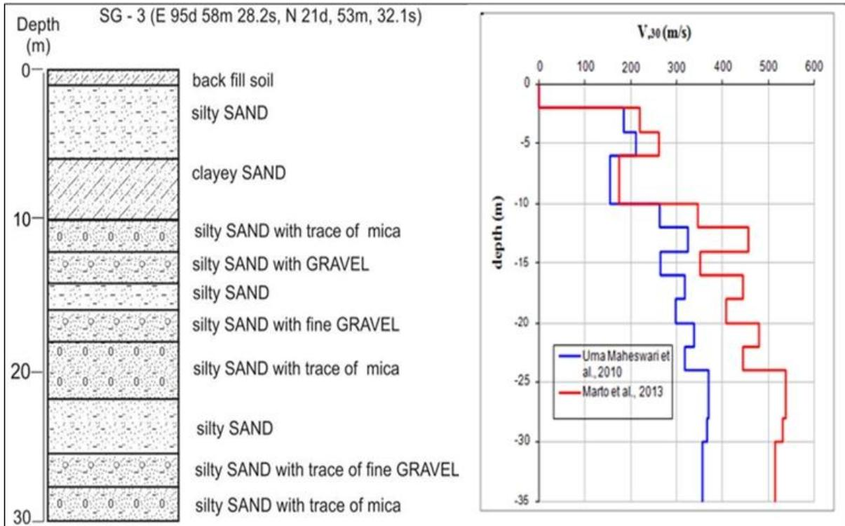
Figure (1.7) Soil profile and shear wave velocity profile ( $V_s 30$ ) by using corrected N value for SG-3
