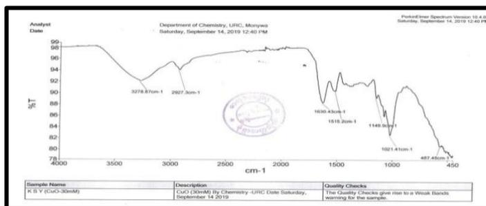
**Figure5. FT-IR Assignment of Copper Oxide Nanoparticles using 30 mM CuSO<sub>4</sub> Solution and Water Rhizome Extract**
