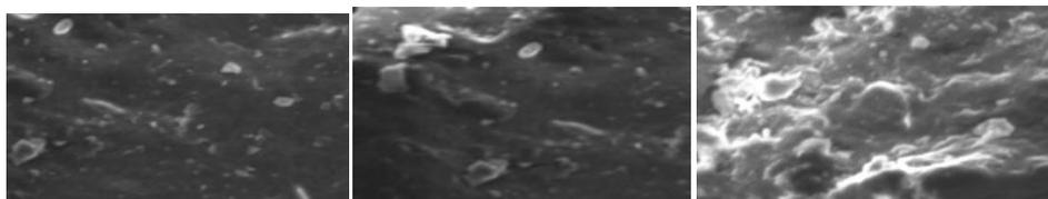
**Figure (4a,4b and 4c) SEM Image of Copper Oxide Nanoparticles using 70, 50, 30 mM of CuSO<sub>4</sub> Solution and Rhizome Extract**
