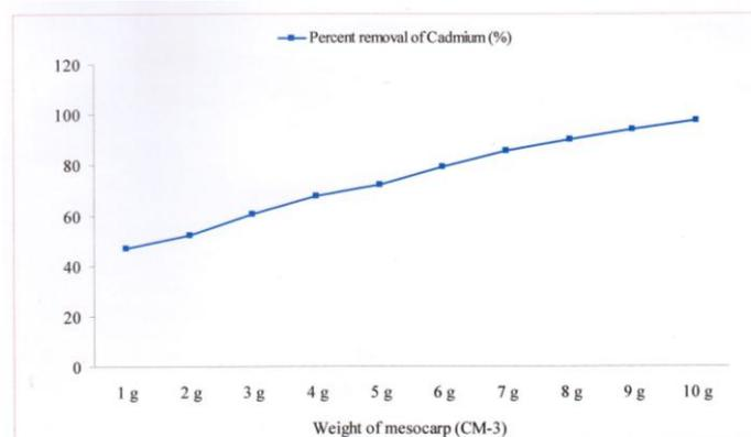
Figure 4. The Plot of Percent Removal of Cadmium by using Various Weights of Mesocarp (CM-3) Sample
