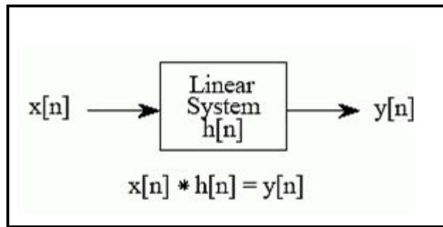
Figure 1. How convolution is used in DSP.
