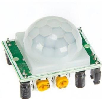
**Fig.5 Photograph of PIR sensor**
