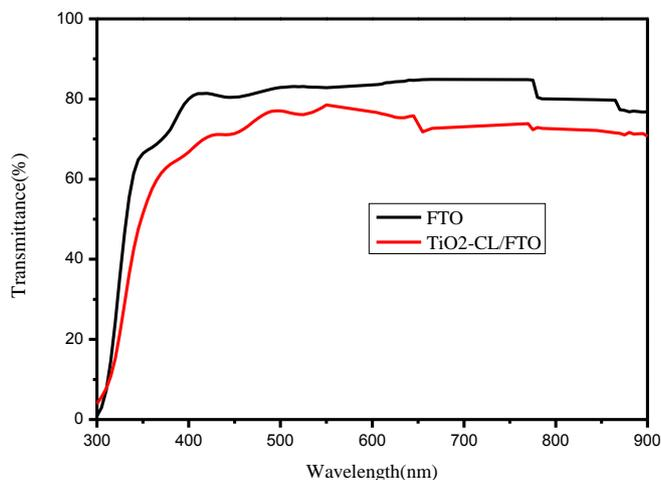
**Figure 2.** The transmission spectra of bare FTO and  $\text{TiO}_2\text{-CL/FTO}$ .
