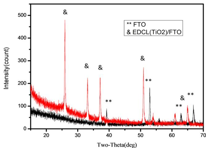
**Figure 1.** XRD spectrum of  $\text{TiO}_2$  compact layer produced from acidic titanium (III) chloride at room temperature following sintering temperature  $450\text{ }^\circ\text{C}$  for 30 minutes. Applied current= $20\ \mu\text{A}$ , deposition time = 1000s.
