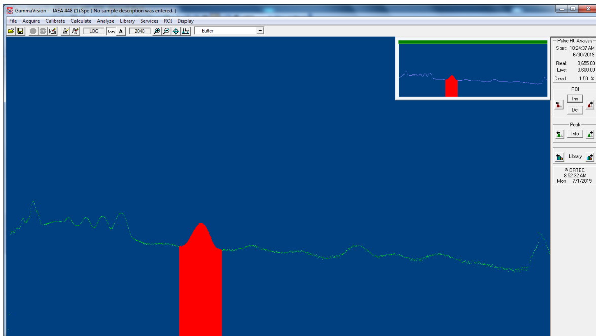
Figure (6) Analyzing the Net Area of an Observed Radionuclide ( ^{214}\text{Bi} at 609 keV) by using Gamma Vision 32 Software
