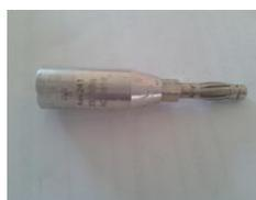
Fig.1.6 Sealed Alpha Source
