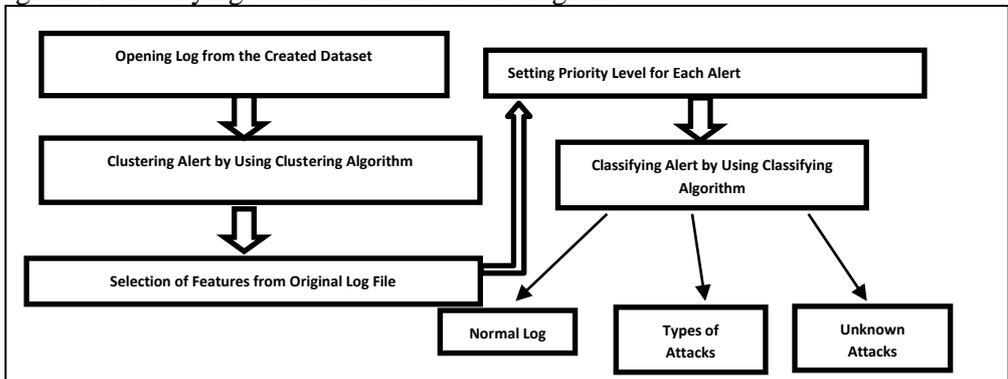
Fig.4 Block Diagram for the Procedures of Classification
