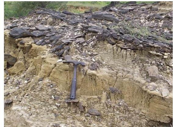
Fig (3.3) Clay, silt and indurated hard sandstone band intercalated in Moza Formation, (near Yebok-chaung)
