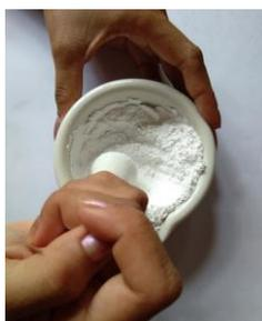
Figure 5 Grinding two samples with agate mortar and pestle
