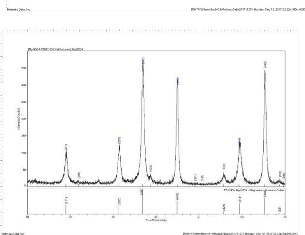
Figure 10 The XRD pattern for MgAl<sub>2</sub>O<sub>4</sub> calcined at 800 °C for 1 hr
