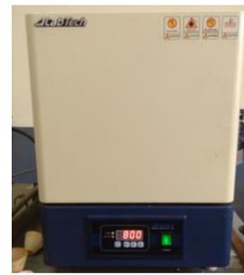
Figure 7 Calcination in electrical furnace at 800 °C for 1 hr
