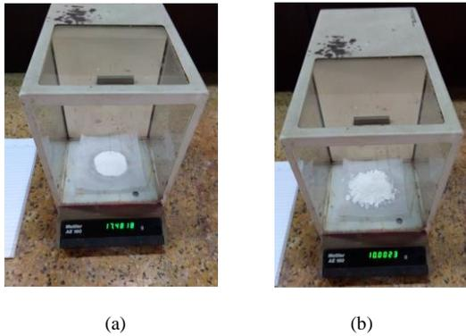
Figure 4 Weighing (a) Al<sub>2</sub>O<sub>3</sub> and (b) Mg(OH)<sub>2</sub> with digital balance
