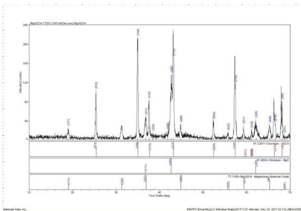
Figure 9 The XRD pattern for MgAl<sub>2</sub>O<sub>4</sub> calcined at 700 °C for 1 hr
