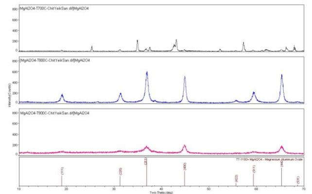
Figure 12 Peaks comparison for MgAl<sub>2</sub>O<sub>4</sub> at 700 °C, 800 °C and 900 °C for 1 hr
