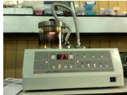
Figure 8 Coating for SEM measurement
