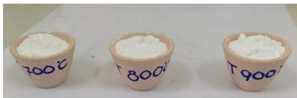
Figure 6 Ground mixtures with crucibles before calcination
