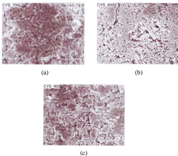
Figure 13 SEM images of  $MgAl_2O_4$  calcined at (a) 700 °C (b) 800 °C and (c) 900 °C for 1 hr
