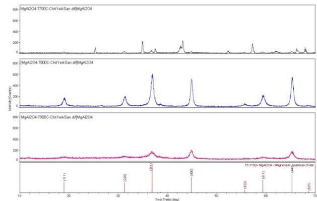
Figure 12 Peaks comparison for MgAl<sub>2</sub>O<sub>4</sub> at 700 °C, 800 °C and 900 °C for 1 hr
