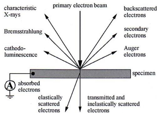
Figure 2 Schematic illustration of the incident electron beam generating different signals in the sample
