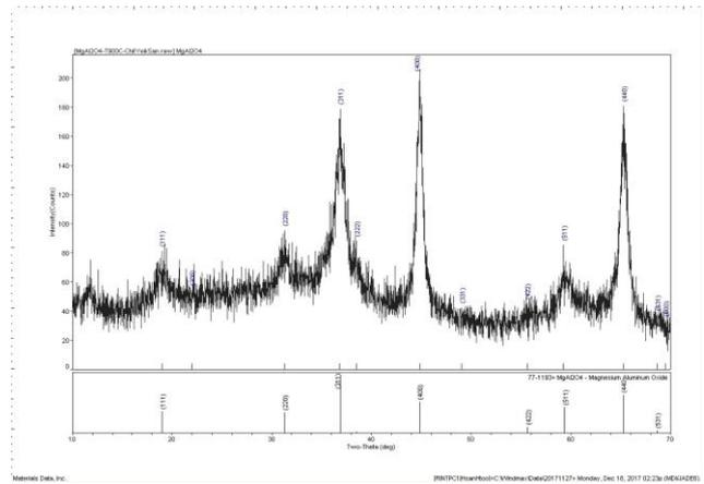
Figure 11 The XRD pattern for MgAl<sub>2</sub>O<sub>4</sub> calcined at 900 °C for 1 hr
