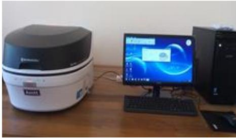
**Figure 6. Photograph of Shimadzu EDX-7000 Spectrometer**
