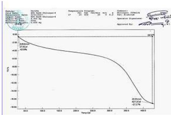
**Figure (13) TG Plots of Extracted Chitosan Deacetylated with 40% NaOH in Nitrogen Atmosphere**
