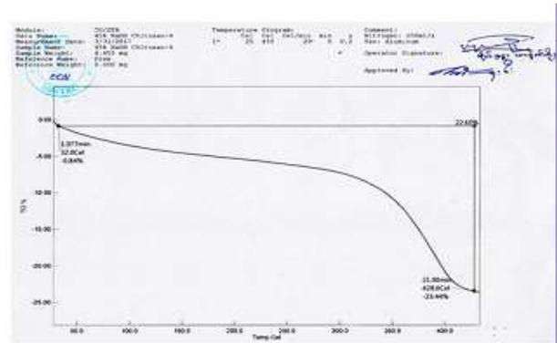
**Figure (14) TG Plots of Extracted Chitosan Deacetylated with 45% NaOH in Nitrogen Atmosphere**
