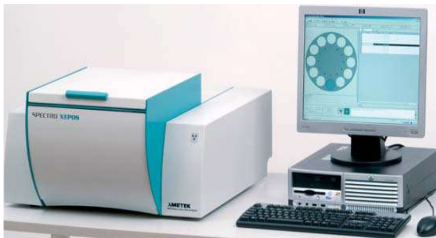
Figure (6) Experimental Set-up for XEPOS Spectrometer Detection System
