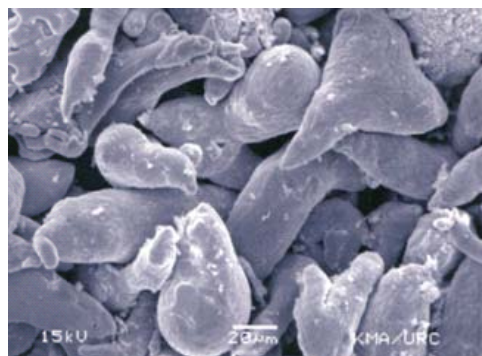
Fig.6. SEM micrograph of aluminum powder at gas pressure 0.5 MPa
