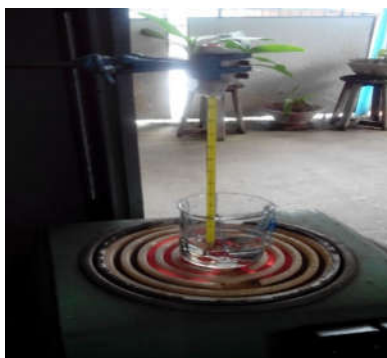
Figure 6. Chemical Etching of SSNTD
