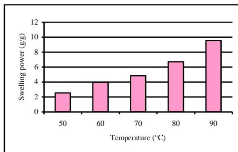
Fig. 6. Swelling Power of Rice Starch with Temperature
