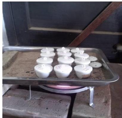
Fig. 5. Determination of Ash Content
