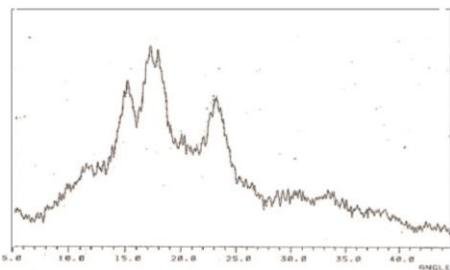
Fig. 8. X-ray Diffractogram of Reference Starch
