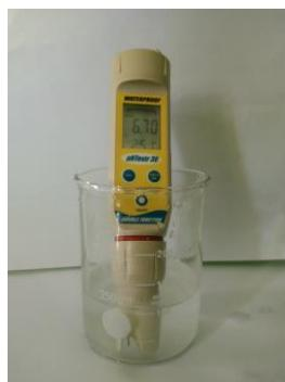
Fig. 3. Determination of pH.
