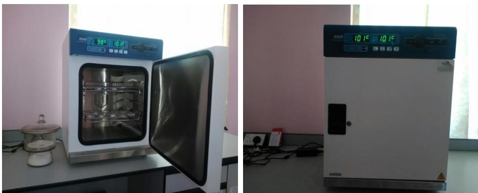
Fig. 4. Determination of Moisture Content
