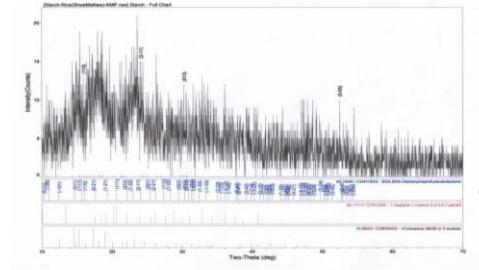
Fig. 9. X-ray Diffractogram of Rice Starch
