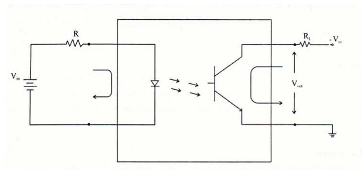
Fig.3 Opto-coupler connected to an external load
