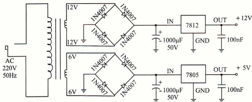
Fig.5 Regulated power supply circuit
