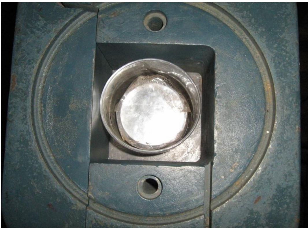
Figure (2) Photograph of top view for sediment sample in the lead shield
