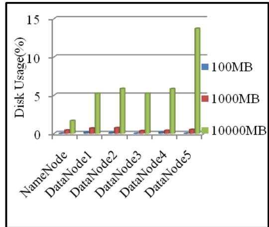
**Figure 7. Average Disk Usage of PC cluster based Storage Server**
