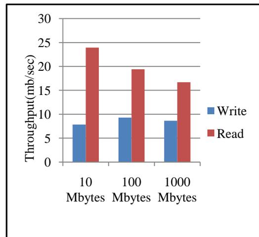
**Figure 8. Throughput of the File Read and Write**
