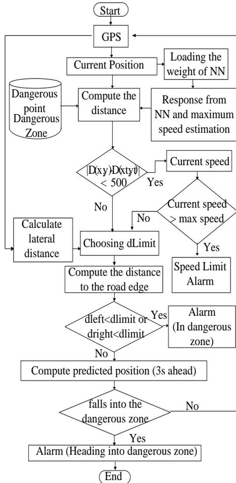
**Figure 2. System flow diagram for intelligent cruise control**
