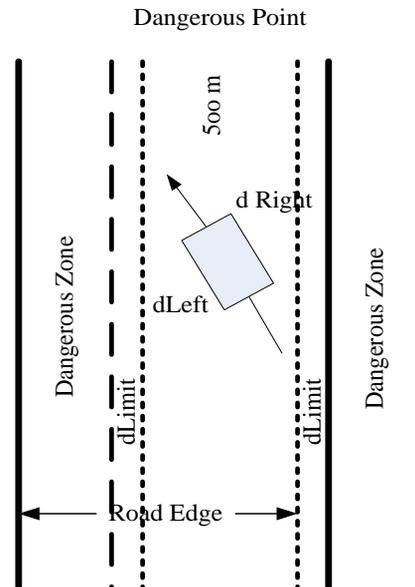
**Figure 1. Dangerous zone, dangerous point and lateral distance**
